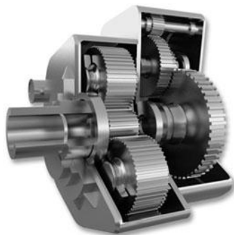
Figure 2 The gearbox converts the 10-15 rpm speed of the rotor to 1500 to 1800 rpm needed for power generation. Photo credit: Timken Co.
